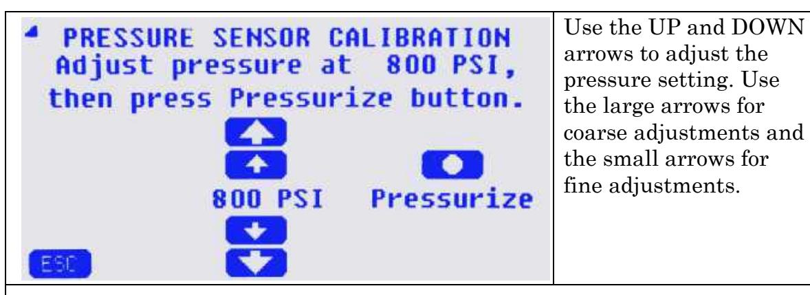
Figure 17 – Adjusting pressure at 80% of max pressure.
