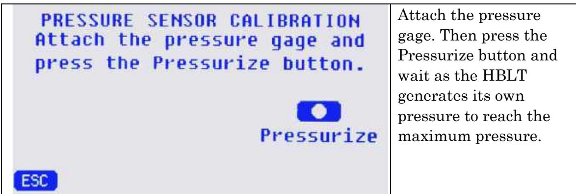
Figure 16 – Pressurizing the HBLT.
