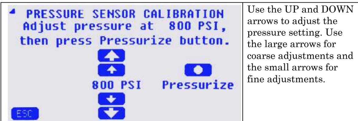
Figure 17 – Adjusting pressure at 80% of max pressure.
