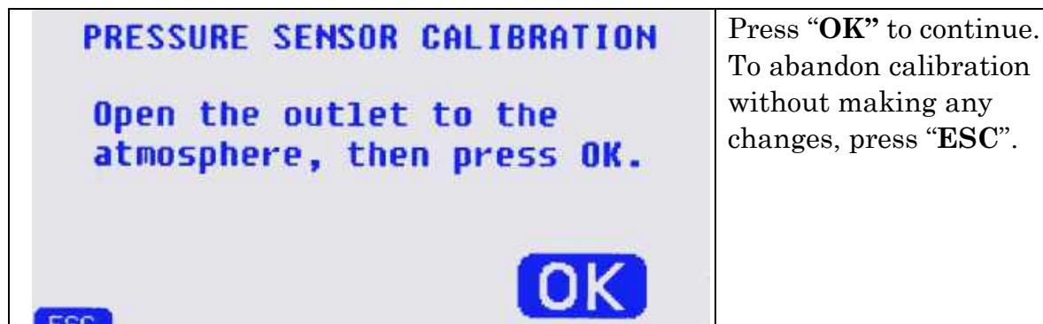
Figure 15 – Setting atmospheric value.
