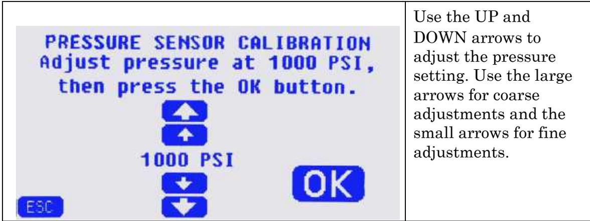
**Figure 18 – Adjusting pressure at max pressure.**
