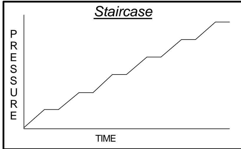
Pressure increases to programmed *Target Pressure* and remains for the *Dwell Time*. If no burst or leak occurs, pressure is then increased by the *Pressure Increment* amount. The test continues until a burst or leak is detected or until *Maximum Pressure* is achieved.
