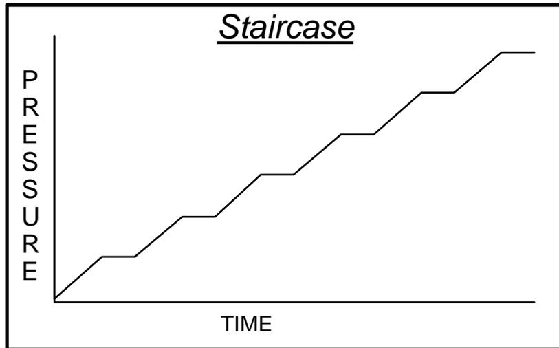
Pressure increases to programmed *Target Pressure* and remains for the *Dwell Time*. If no burst or leak occurs, pressure is then increased by the *Pressure Increment* amount. The test continues until a burst or leak is detected or until *Maximum Pressure* is achieved.
