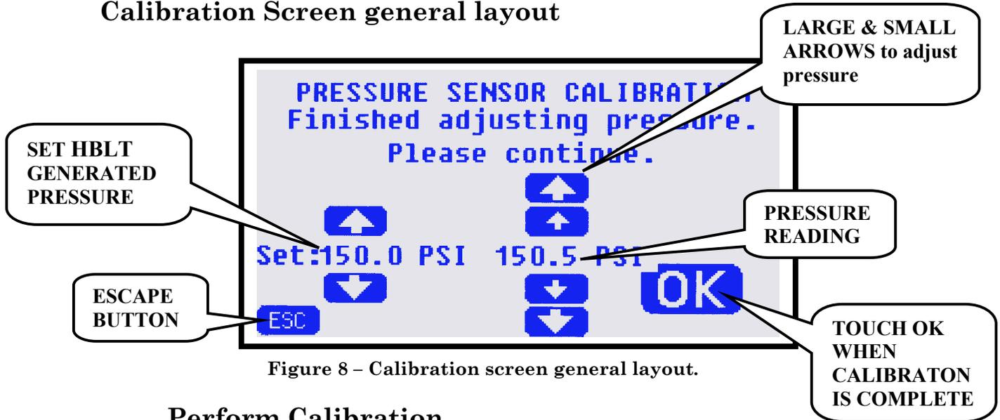
Figure 8 – Calibration screen general layout.
