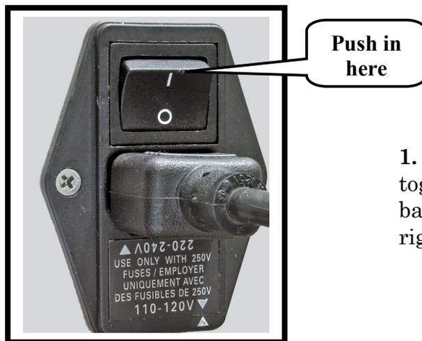
1. Turn On Power – push the toggle switch located on the back of the machine, exterior right, to the “Up” position.
