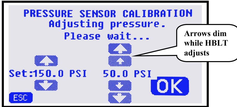
Figure 22 – Waiting for the new pressure target.
